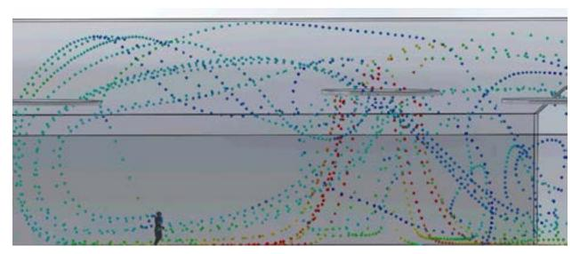
Using advanced fluid dynamics modeling, the movement of air and de-stratifying effects of HVLS fans are visible.
