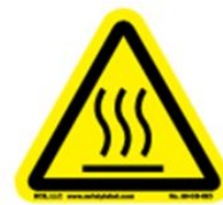
Burn Hazard / Hot Surface
