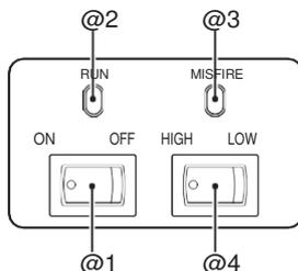
When the flame is extinguished, turn "OFF" the operating switch.
