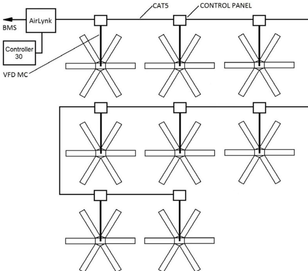
\*AirEffect is not compatible with Dual Control. Temperature monitoring by BMS can regulate fan operation.
