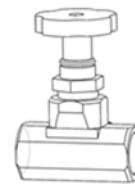
Fire Stop Valve Closed
