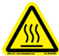
Burn Hazard / Hot Surface
